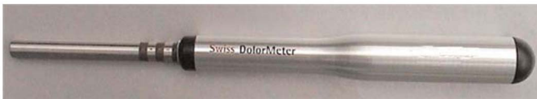
Figure 2: Dolormeter for the application of a defined pressure of 0-50 N. Pressure is applied over a circular area of 1 cm.
